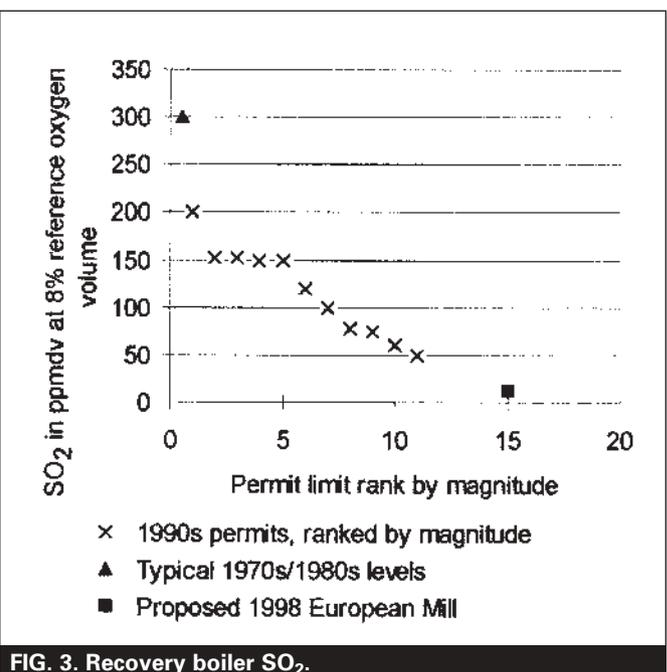
FIG. 3. Recovery boiler SO<sub>2</sub>.
