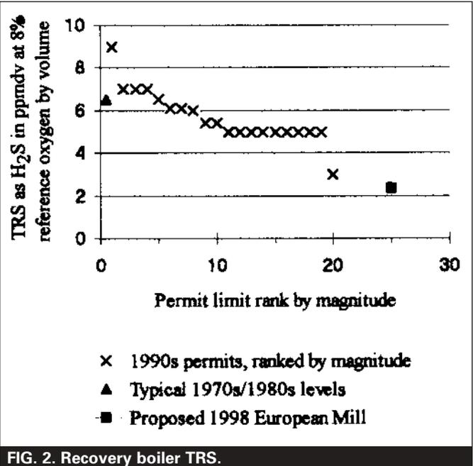
FIG. 2. Recovery boiler TRS.
